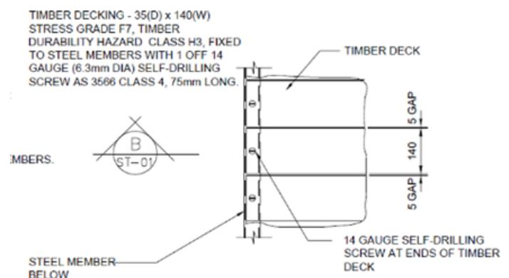
The platform must be in contact with greater than 95% of the area of the base of the tank with gaps of 5 mm (preferred) but no greater than 25mm between supports.
